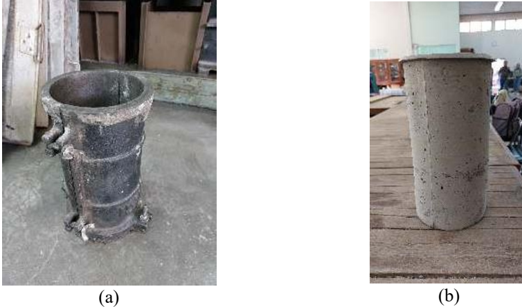
Fig. 4. (a) Test specimen mold 15 x 30 cm (b) The specimen.
