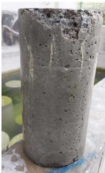
Fig. 6. Specimen contain 2% capsule after compressive test and curing.
