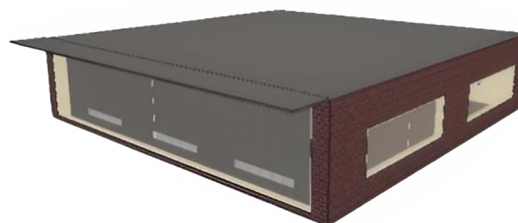
Fig. 1. 3D view of a building integrated with a Trombe wall.
