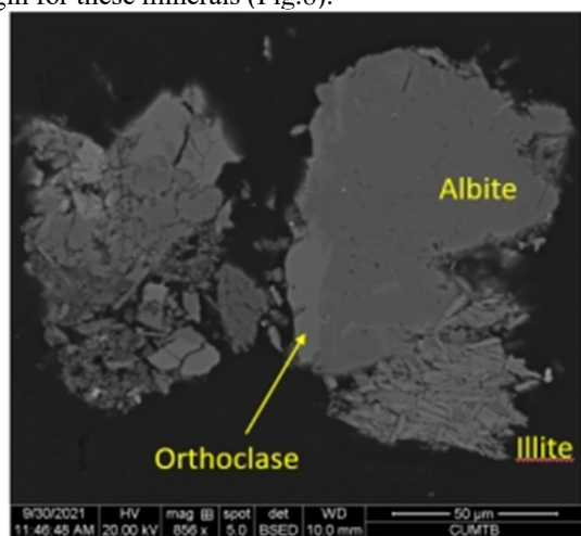
Fig. 8 Albite and orthoclase, under SEM, back scattered image
