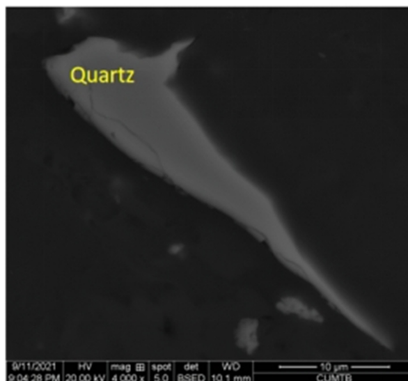
Fig. 2 Quartz: fracture-infillings, under SEM, back scattered image
