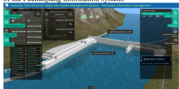
FIG. 1. Homepage of Fuchunjiang system (The homepage features a 3D baseboard displaying the power station and geographical scene, partially achieving a digital twin. The dashboard shows important design parameters and real-time monitoring data of the gates. Additionally, it is equipped with tools for alarm alerts and video surveillance.)
