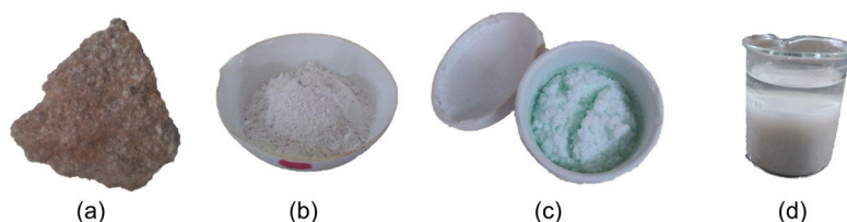
Fig. 2. a) pyrophyllite (raw material), b) pyrophyllite powder, c) calcined-alkali fusion pyrophyllite, d) precipitated silica from Pyrophyllite.
