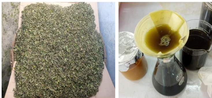
Fig. 4. Drying Process of Moringa Leaves into Powder (left), Filtration Process of Macerated Moringa Biosurfactant Results (right).
