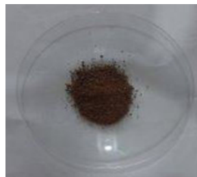
Fig. 12. Sodium Lignosulfonate with 75 Minutes Reaction Time, 450 W Power, and 0.3 M NaHSO 3 Concentration
