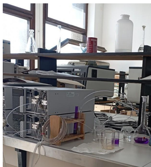
Fig. 1. Experimental set up, PTFE microreactor tube is connected to two plunger pump units
