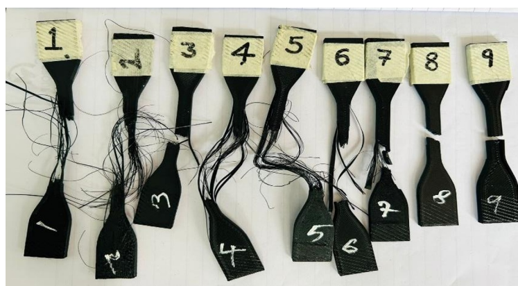
Fig.8 PETG Tested Tensile specimens (ASTM D638)
