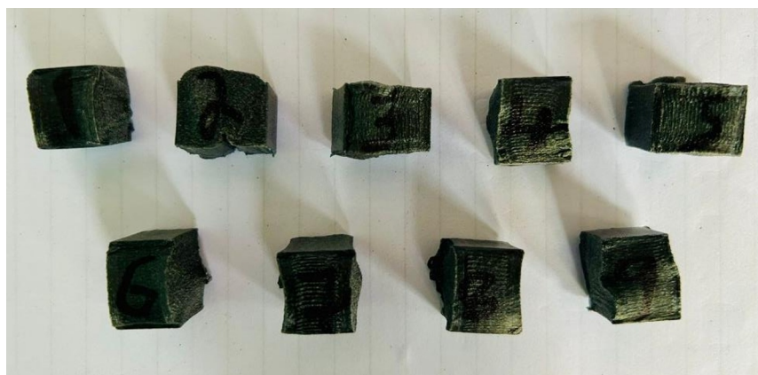
Fig.9 Carbon fiber-reinforced PETG Tested Compressive specimens (ASTM D695)
