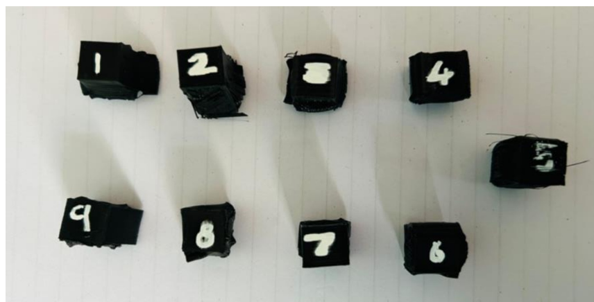
Fig. 10 PETG Tested Compressive specimens (ASTM D695)
