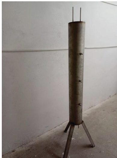
Fig. 5. Experimental installation for testing methane displacement by hydrogen.
