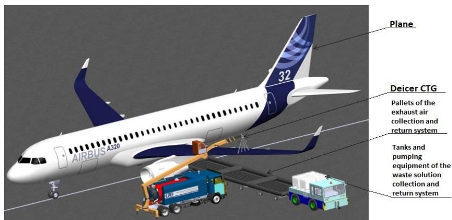
Fig. 3. KNO-AERO-MA complex for processing (washing, anti-icing protection) of external surfaces of aircraft.
