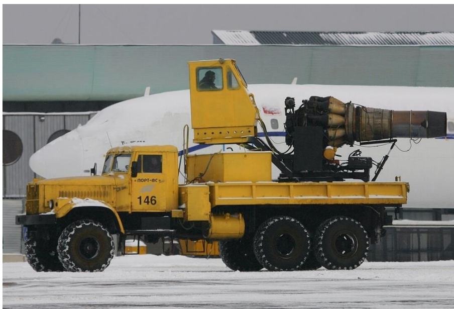
Fig. 1. MAZ car with an old jet engine from an airplane installed.
