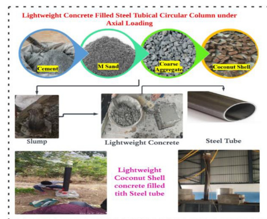
Fig 1: Overview of the CFSTC under axial loading
