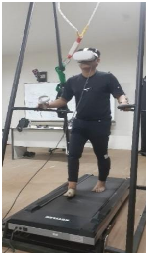
Fig. 1. A visual display of walking simulation on a VR-based prosthetic gait training system
