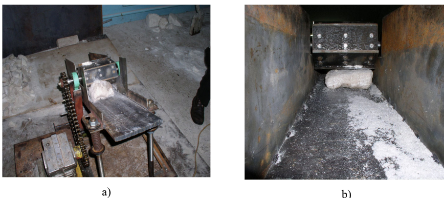
Fig. 2. Destruction of caked material: a) sharp-pointed blades of the drum; b) the edges of the drum blades.
