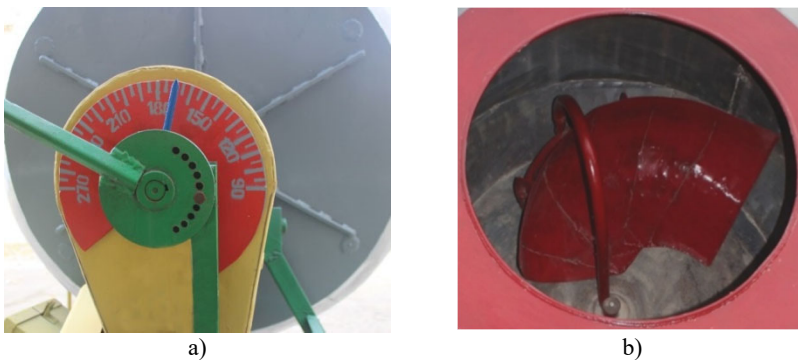
Fig. 2. a) The appearance of the shovel's installation in relation to the horizontal axis. b) The view of the shovel inside the drum.
