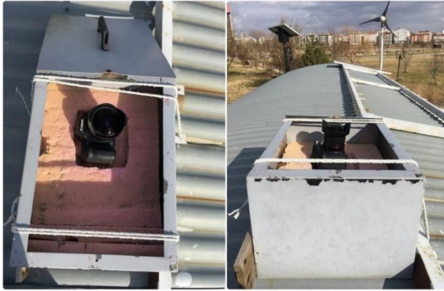
Fig. 1. Sky imaging system placed on the roof of Afyon Kocatepe University Solar and Wind Application and Research Center (GÜRAM).
