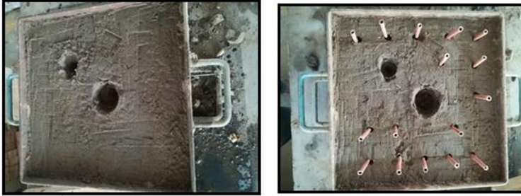
Figure 2 (a) Without copper tube (b) With copper tube
