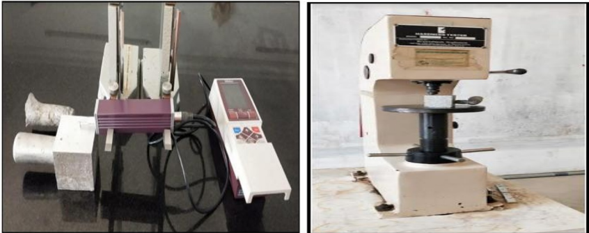
Figure 6. (a) Surface Roughness tester, (b) Brinell Hardness Test Machine
