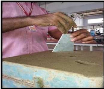
Figure 3 (a) 90° vent hole (b) 60° vent hole (c) 45° vent hole
