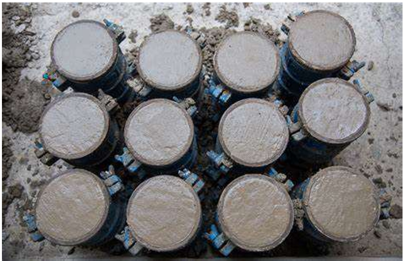
Figure 7: Casting of Cylinder Specimen
