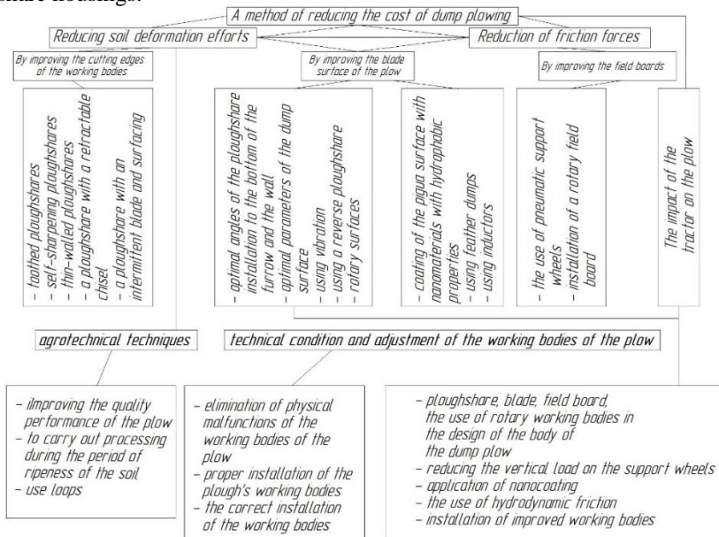
Figure 1. A block diagram of possible methods for reducing energy costs for plowing
