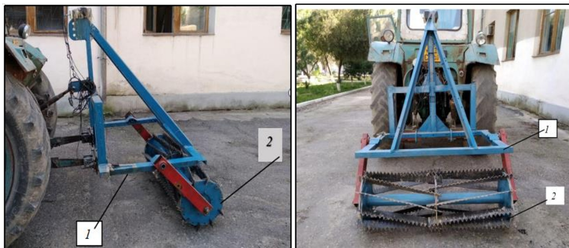
Fig. 2. Side (right one) and rear (left one) views of the laboratory-field device, (1) frame suspension device; (2)-roller
