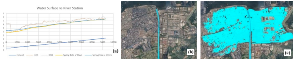
Fig. 4 (a) 1D flood modelling in existing condition; (b) 2D flood modelling in scenario 4; (c) 2D flood modelling in scenario 5
