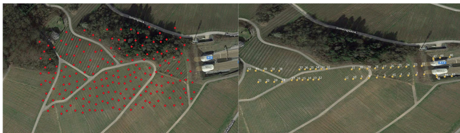
Fig. 1. On the left: Seismic network on the surface. On the right: Seismic network in the tunnels. The red and yellow dots represent the location of the seismic nodes.
