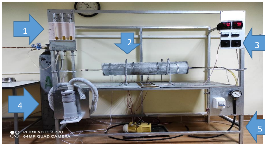
Fig. 1. Unit for the synthesis of multi-walled carbon nanotubes (MWCNT). 1- gas raw material production unit: gas raw material (propane, butane, their mixture) is diluted with argon to the required thickness and fed to the reactor zone at a certain speed. 2- the reactor unit consists of 2 sections of a tube furnace with a quartz reactor inside, each with independent heating. The furnace heats the reactor up to a temperature of 1000°C. 3- the temperature regulation section of the furnace consists of a temperature regulator that automatically controls and maintains the set temperature in the reactor and two regulators for supplying current to the coil of the furnace. 4- air conditioning unit. 5- vacuum block: the block for creating a vacuum in the reactor is designed for the synthesis of MWCNT at reduced pressures (80-20 kPa). The unit consists of a vacuum pump, a valve and a manometer.
