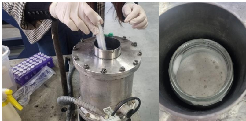
Fig. 2. Sampling from the working area of a plant with a discrete secondary part
