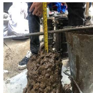
Figure 5. Geopolymer Concrete Slump Test Results
