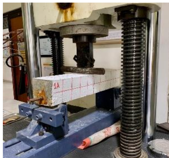
Fig. 4. Flexure test scheme
