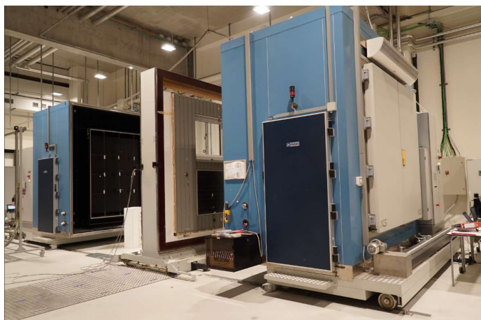
Fig. 2. “Multifunctional façade lab”. From the left: hot chamber with inside the metering box, frame to hold the sample with a sample installed, and cold chamber with openable back side (white doors) to add the sun simulator (© Eurac Research - Annelie Bortolotti).
