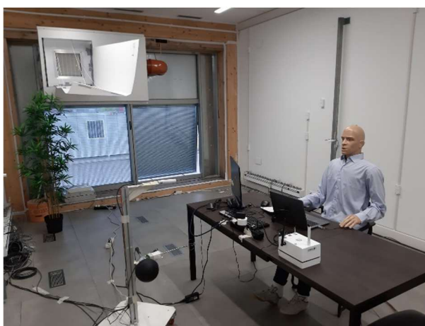
Fig. 5. Thermal manikin. Preliminary tests in the “Façade system interaction lab” to enhance the set-up for human participants within H2020 MEZeroE experimental studies.
