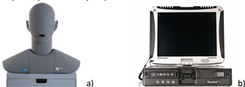
Fig. 6. “Head and torso” simulator with artificial ears and mouth (a) and sound level meter and analyser (b).
