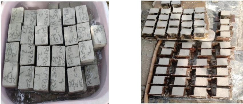
Fig 2. Cubes for testing
