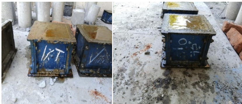
Fig. 4. Casting of cubes with 0.5% and 1% Turmeric powder
