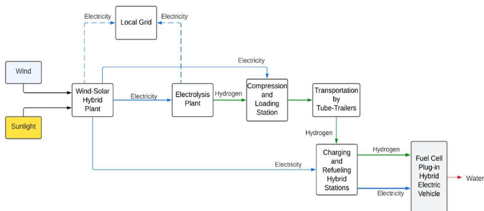
Fig 1. Model to integrate green Hydrogen to power Fuel Cell Plug-in Hybrid Vehicles
