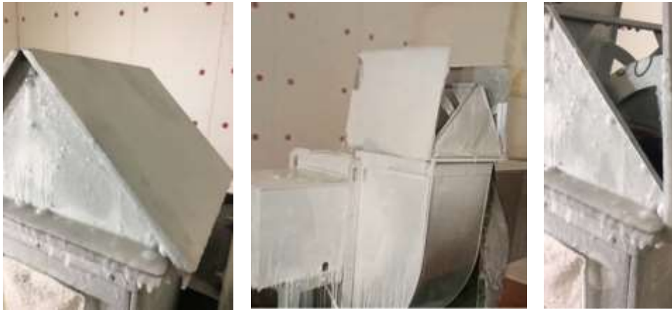
Fig. 6. Checking the operability of the flare system when simulating an ice rain.
