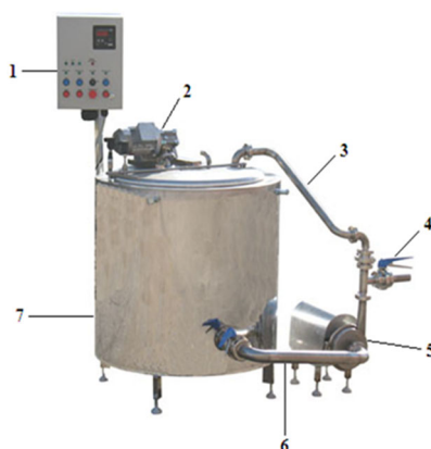
Fig. 1. Laboratory installation for mayonnaise production 1- control device, 2- mixing device, 3, 5, 6- nozzles, 4- faucet, 7- tank.
