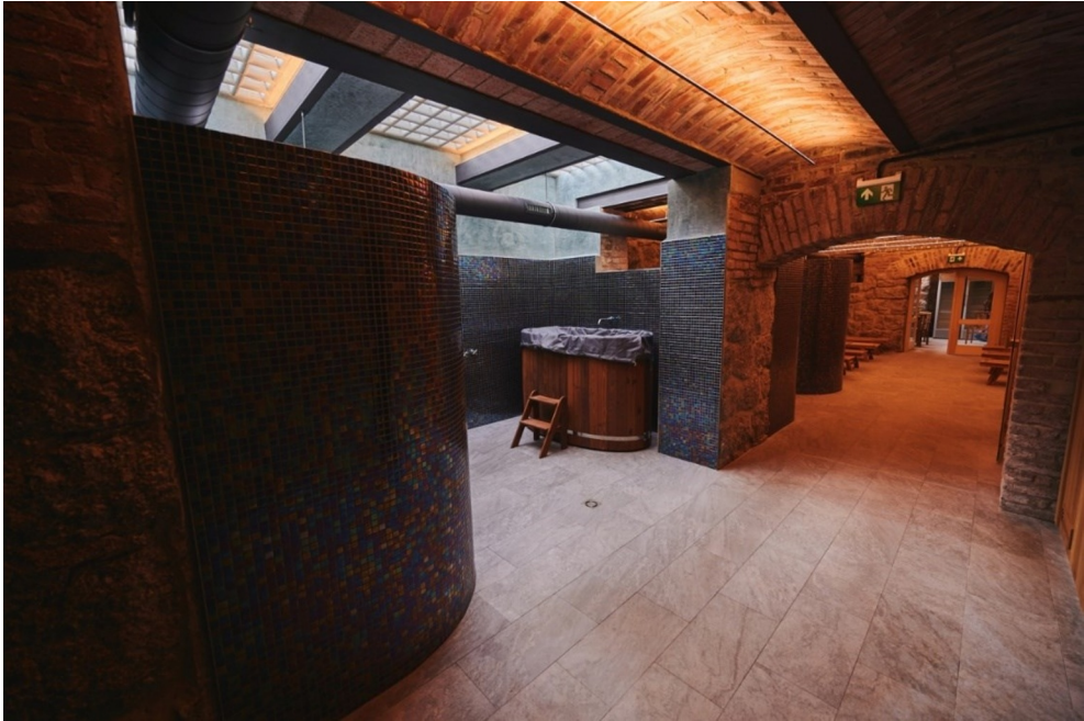
Fig. 5. Underground space illumination through glass fittings in the ceiling [11].
