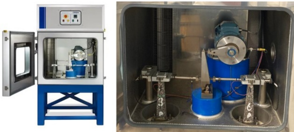
Fig. 6 COOPER CRT-2PT-FET (on the left the whole device, on the right a detail of the inside of the device and mounted samples).
