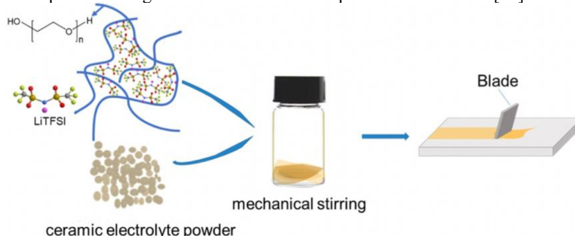
Fig. 1. Manufacturing process of PEO/LGPS composite electrolyte [13].
