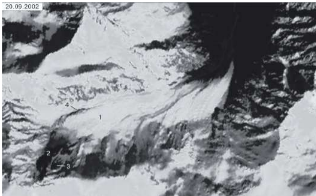
Fig. 3. The Kolka Glacier's circus 8.5 hours before the disaster on 20 September 2002 on satellite images Landsat 7 ETM+ 1 – The Kolka Glacier; 2 – the zone of collapsed rocks; 3 – the place of the hanging glacier, which collapsed in the period from 19 August to 20 September 2002; 4 – the shadow of the ledge of the glacier surface
