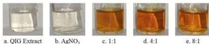
Fig. 1. Colors of Solution (a) QIG Extract, (b) \text{AgNO}_3 , Ratio of \text{AgNO}_3 /QIG Extract (c) 1:1, (d) 4:1, (e) 8:1.
