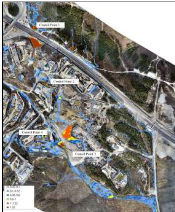
Fig. 4. Scheme of flooding of the territory, main waterlogged zones at high intensity of 1% precipitation without the designed collector.
