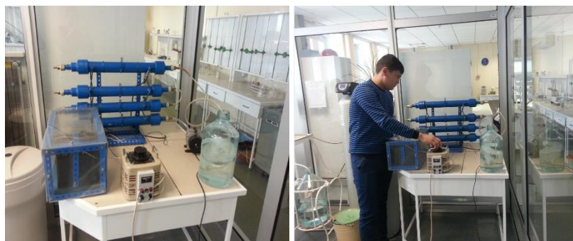
Fig. 1. The ETRO - 02 laboratory ozonator device based on electric corona discharge ( the ozonator device is protected by a copyright certificate "Patent No. 83218 Ministry of Justice of the Republic of Kazakhstan - 2014" ).
