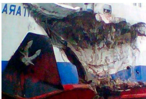
Fig. 6. Structural damages due to collision experienced by passenger carrier [6].
