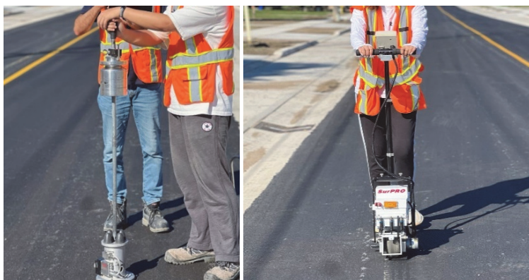
Fig. 3. Light Weight Deflectometer (Left) and SurPro Equipment (Right)
