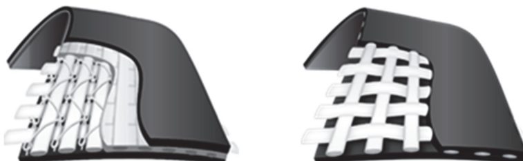
Figure 4: An image of a warp-knit reinforced membrane is shown on the left. It has a narrow stitch yarn that binds the perpendicularly oriented and heavier warp and fill yarns. The warp-knit is encapsulated with an adhesive layer that bonds the polymer facecoats to the textile reinforcement. This is shown as the translucent middle layer in the left illustration. A membrane with an open weave reinforcement is shown on the right.
