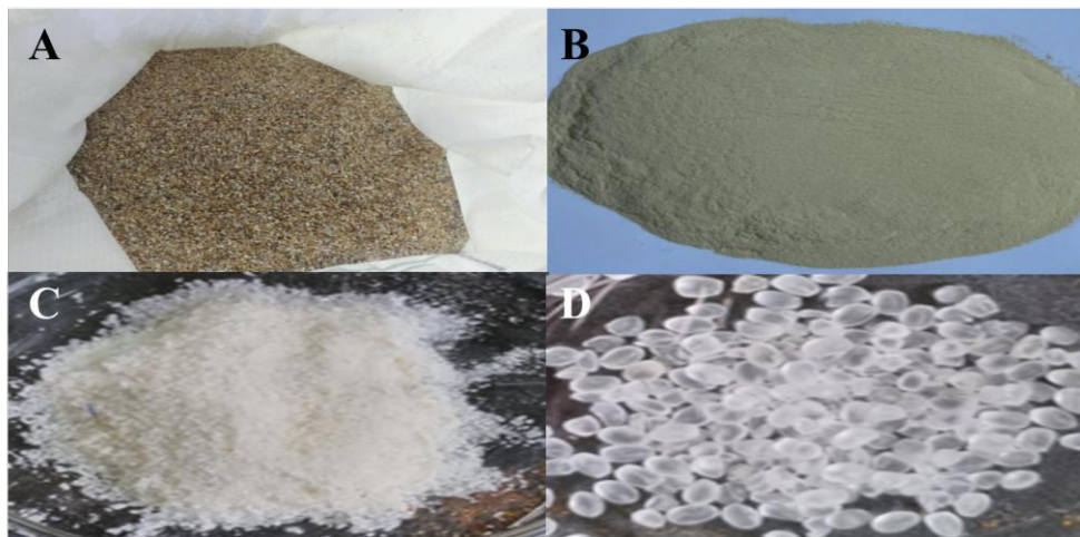
Figure 1. Materials used in this study; A: Ottawa sand, B: Organo-bentonite, C: Polynorbornene, D: polyolefin
