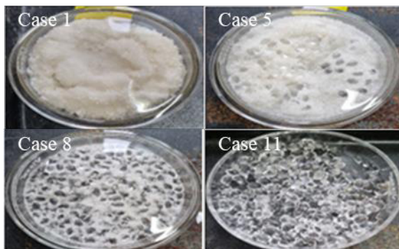
Figure 6. The swelling effect of the polymer 120 minutes after contact with TCE
