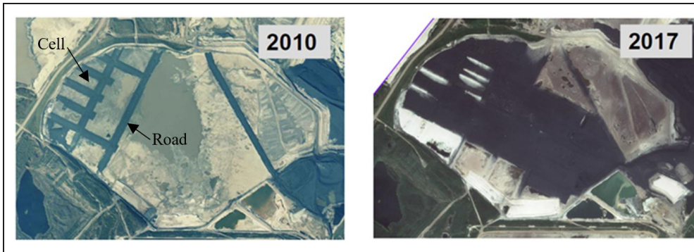
Fig. 1. Coke cover with part of the road network in 2010 and the completed 2 m cover in 2017
