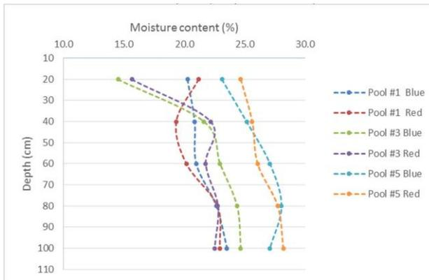
**Fig. 7.** Moisture content in depth-Pool #1, 3, and 5
