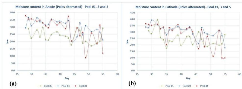
**Fig. 5.** (a) Moisture content in Anode-Pool #1, 3, and 5, (b) Moisture content in Cathode-Pool #1, 3, and 5.
