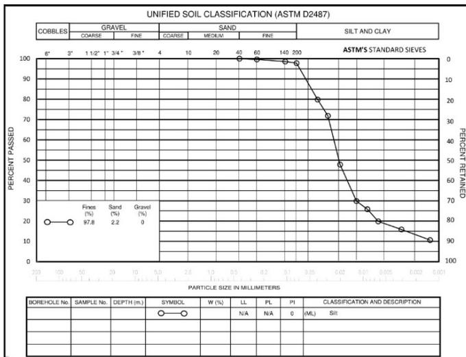
**Fig. 2:** Unified Soil Classification Curve of the Tailing Utilized in this Study
