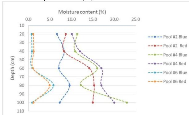
**Fig. 8.** Moisture content in depth-Pool #2, 4 and 6
