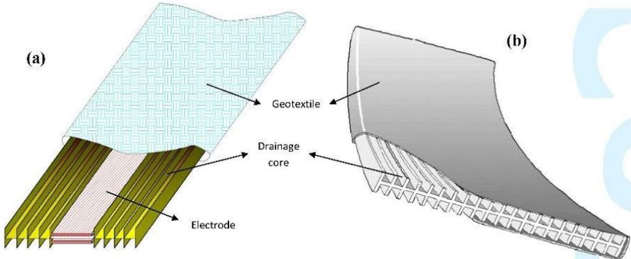
**Fig. 1.** (a) Patented drainage media (wick drain and electrode) (b) original CeTeau's wick drain.
