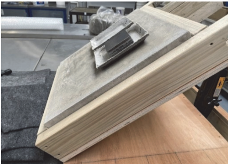
Fig. 3. GCCM-PVC specimens on concrete slab
