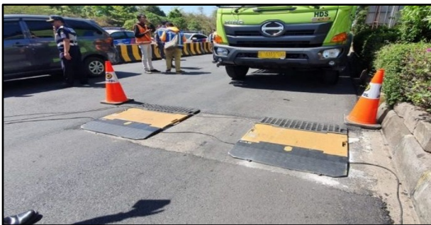
Fig. 4. Vehicle weight measuring tool using weight in motion
