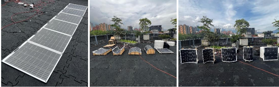
Figure 4. Experimental setup. Left: Flat panels. Center: Horizontal position. Right: Vertical position
