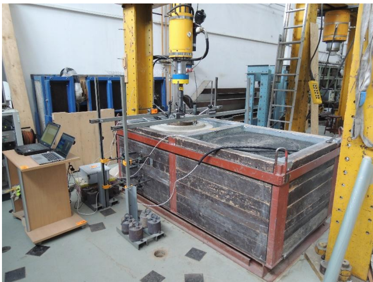
Fig. 3. An overall view of the experimental box during the static plate loading test.
