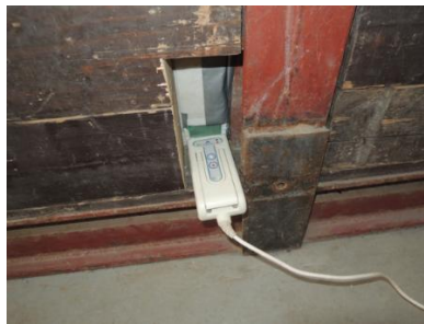
Fig. 6. Hole for the extended tail of the pressure mapping sensor to capture data.
