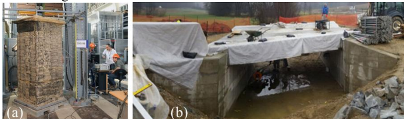
Fig. 2. (a) Large-scale testing (b) Construction of GRS abutments adopted from Lenart et al (2016) [15]
